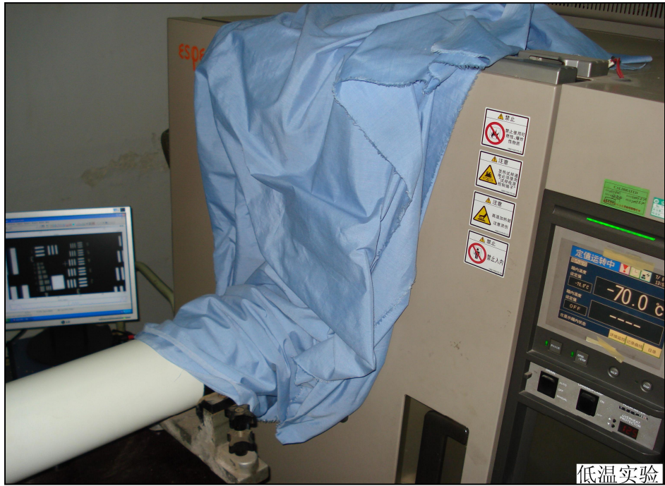
Fig.4 CSTAR winterization test
