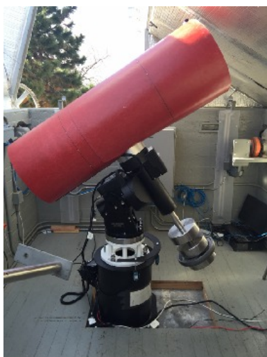
(a) Telescope mount with a simulated payload.
