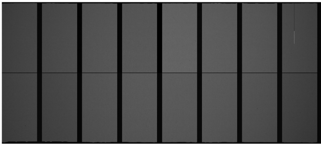
Figure 4. A 10\text{k} \times 5\text{k} flat-field image for one CCD camera, showing the 16 read-out channels. The black gaps are 180-column horizontal and 10-line vertical overscan regions for each channel – there are no gaps on the sky.
