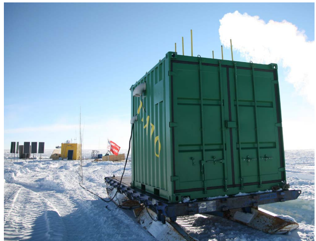
FIG. 3. (Color online) Picture of PLATO installation at Dome A. The (green) engine module is shown in the foreground. In the background the solar panel array and the (yellow) instrument module can be seen.
