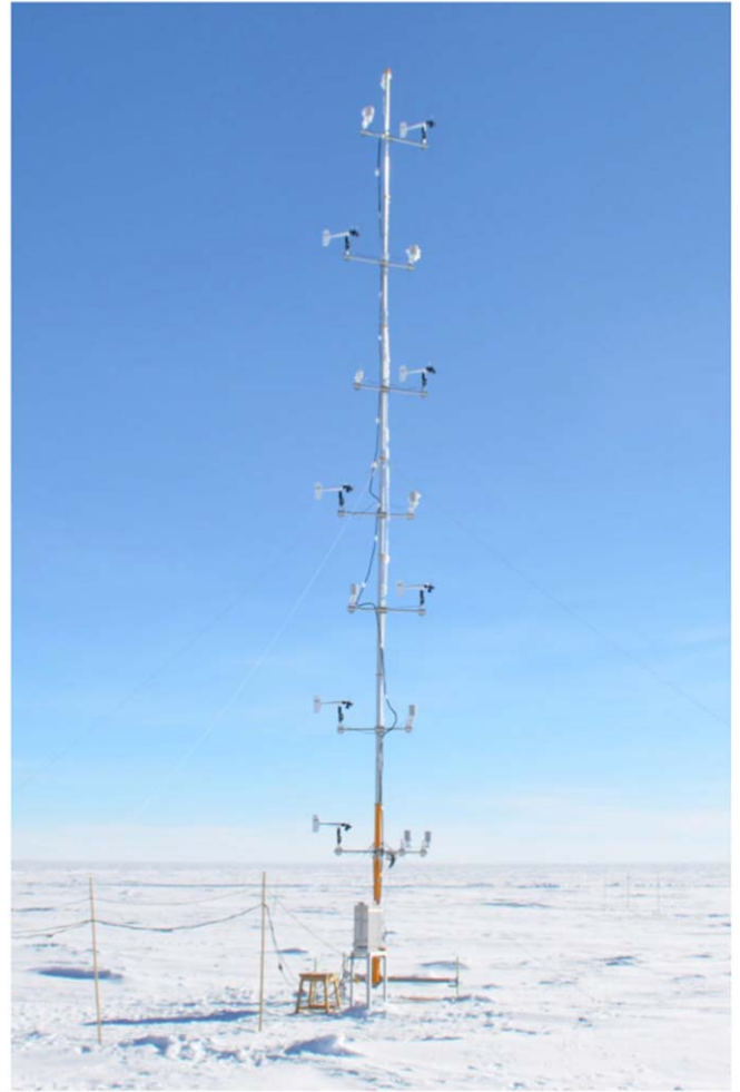
Figure 1. KLAWS-2G installed at Dome A in 2015 January. The temperature sensors (in the radiation shields) and anemometers are clearly visible. The electronic box sits at the foot of the mast. The photo was taken in 2016. (A color version of this figure is available in the online journal.)
