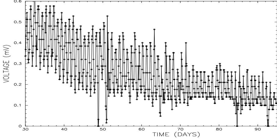
**Fig. 3.** Full COBBER data set from January to April 2003. Even without removing the diurnal variations caused by the sun heating the instrument, the four recorded days of cloud ( $V_{signal} = 0$ ) are clearly seen.
