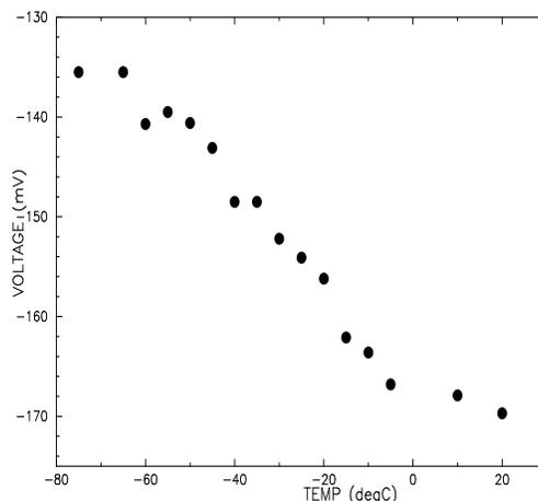
**Fig. 2.** Signal voltage of TPS534 detector for a source  $15^{\circ}\text{C}$  warmer than ambient, versus ambient (Detector) temperature.
