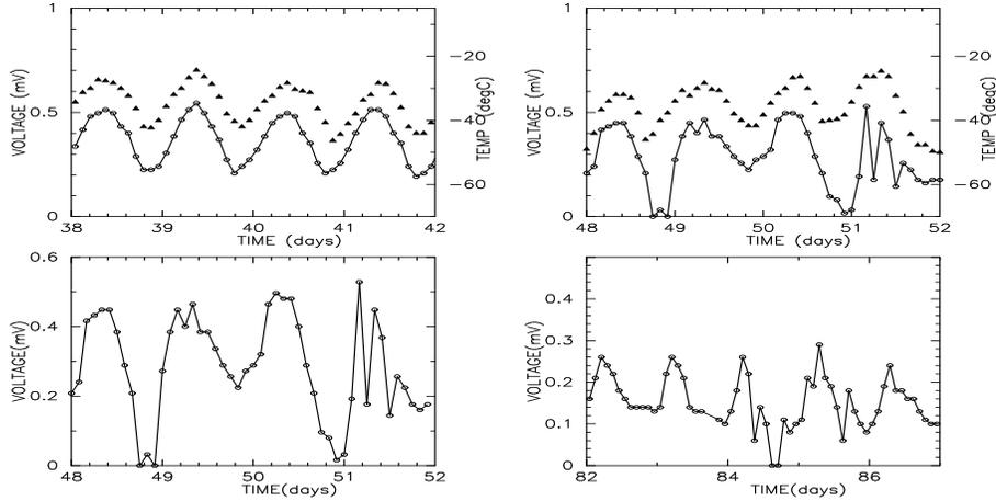
**Fig. 4.** Top Left: Four clear days (solid line) and  $T_{ambient}$  (triangles). Top Right: Two cloudy days (solid) and corresponding  $T_{ambient}$ . Bottom Left: Signal strength in February and Bottom Right: Early April. Overcast conditions are still detectable.
