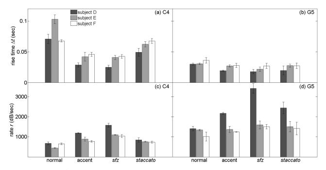
FIG. 8. The averaged rise time  $\Delta t$  and the rate *r* of exponential increase in the fundamental  $p_1$  for normal, accented, *sforzando*, and *staccato* notes played by each of the three experts. (a) and (c) show the values for the written C4 note, (b) and (d) for the written G5 note. Bars with different shading represent the three expert subjects. Vertical lines show standard deviations.
