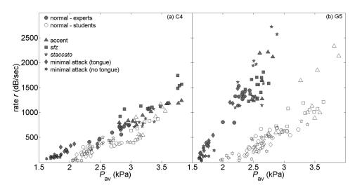
FIG. 12. The rate *r* of increase in fundamental  $p_1$  versus  $P_{av}$  for normal, accented, *sforzando*, *staccato*, and minimal attack notes with and without tonguing played by experts (grey) and students (white), (a) C4 and (b) G5 notes. Different symbols indicate different articulations.
