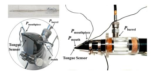
FIG. 1. (Color online) Photograph of the clarinet reed, mouthpiece, and barrel modified to measure tongue contact, mouth pressure, mouthpiece pressure, and barrel pressure during performance. The circular inset at bottom left shows a close-up of the mouthpiece tip, where the tongue sensor (reed with a wire glued on its axis) and the two pressure transducers are visible. A photo at top left shows the modified reed.
