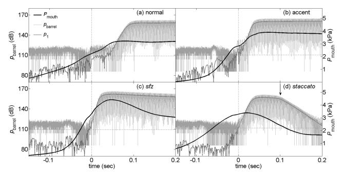
FIG. 5. The slowly varying (DC) component of the mouth pressure  $\bar{P}_{mouth}$  (black), and the amplitude (RMS) of the fundamental  $p_1$  (dark grey) extracted from the barrel pressure  $p_{barrel}$  (light grey) for different articulations for the written C5 notes played by subject D. In each example the horizontal dashed line indicates the noise level in the barrel in dB calculated over the 0.1 s before tongue release.
