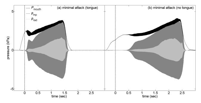
FIG. 11. Measured mouth pressure  $P_{\text{mouth}}$  (black), mouthpiece pressure  $p_{\text{mp}}$  (dark grey), and radiated sound  $p_{\text{rad}}$  (light grey) as functions of time for typical examples of minimal attack (a) with tonguing and (b) without tonguing of the written C5 note, as played by subject D (one of the expert players). t=0 is defined as the instant when the tongue breaks contact with the reed.
