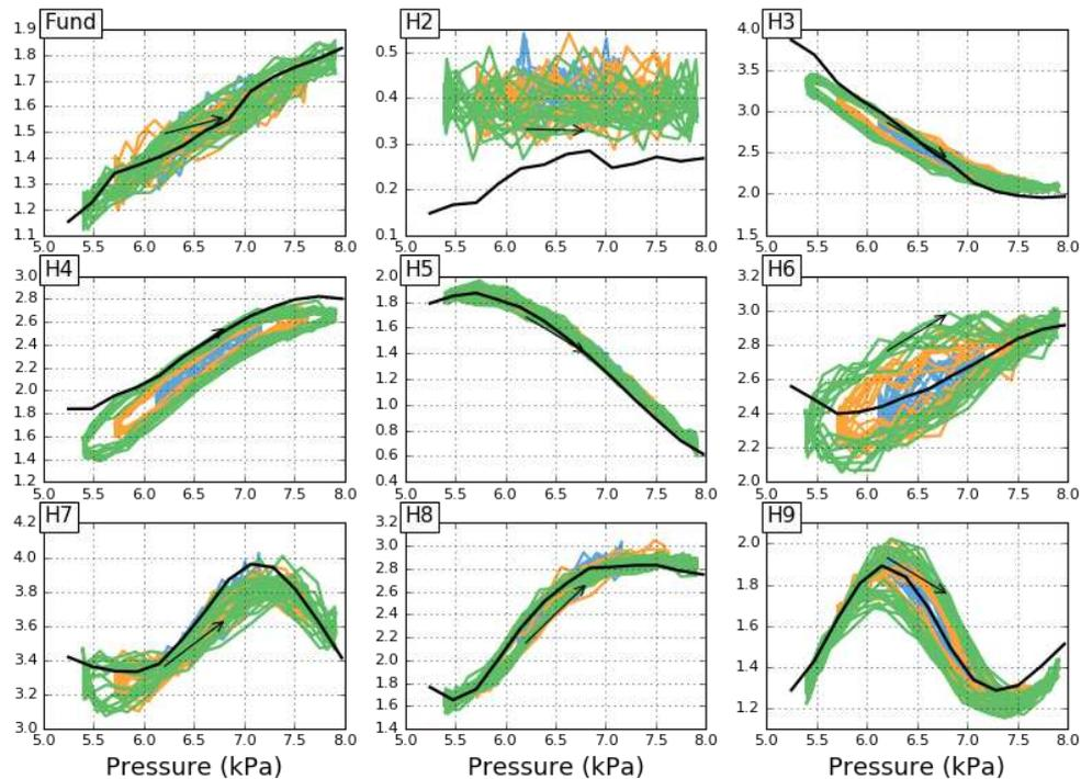
Figure 6 Amplitude in Pa of partials obtained in the 3 vibrato signals, plotted against the instantaneous mouth pressure. For comparison, the amplitude corresponding to the steady state for the blowing pressure value is shown as a thick black line. The plotting range in the amplitude axis is adjusted for each partial. Notice that the 2<sup>nd</sup> partial exhibits a much smaller range than the others.
