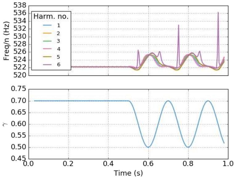
Figure 8 Time course of the frequencies of partials of the signal simulated with the mouth pressure profile shown in the previous figure. Each frequency is divided by its harmonic number
