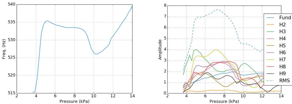
**Figure 3** Fundamental frequency (left) and amplitude [Pa] of harmonics (right) plotted against blowing pressure. RMS amplitude is included for comparison. Amplitudes are obtained from signal radiated near the bell of the oboe
