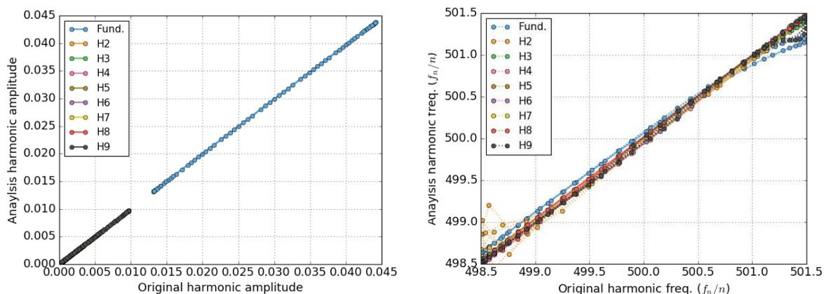
Figure 2 Estimated vs original partial amplitudes and frequencies
