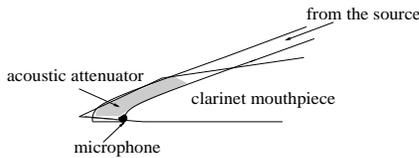
Figure 2: Scheme of the measurement head
