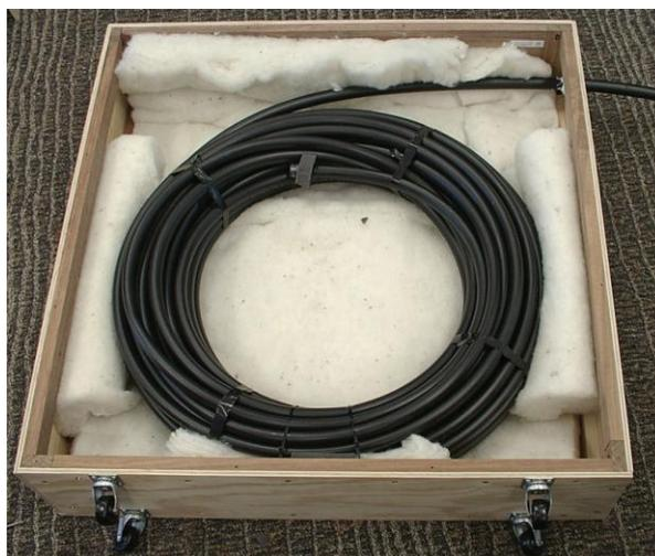
**Figure 3:** The portable infinite waveguide built by ResMed for calibration of and verification of acoustic testing procedures. The timber box is 800 mm square and 210 mm deep.
