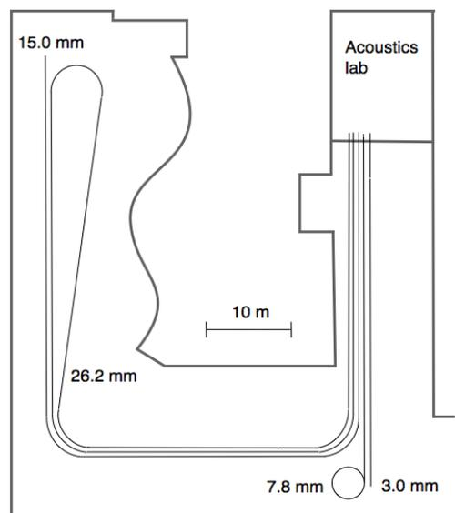
**Figure 1:** A plan of the physics building at UNSW, showing the acoustics laboratory and the 'infinite' waveguides installed in the ceiling space. The 7.8 mm guide is terminated with a 100 m coil. The 26.2 mm guide has both ends accessible in the laboratory.
