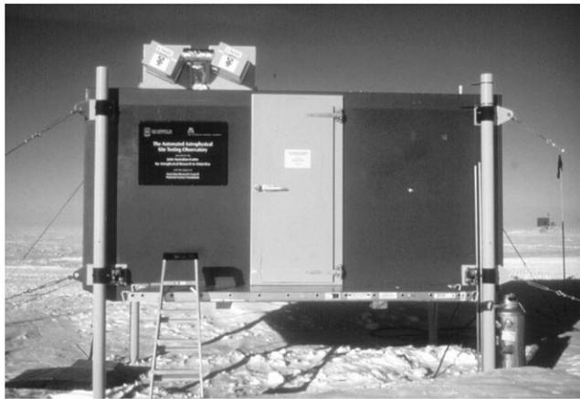
FIG. 1.—AASTO at the South Pole in 1997 January. The left-hand small box on top of the AASTO is the NISM; the box on the right is the MISM.
