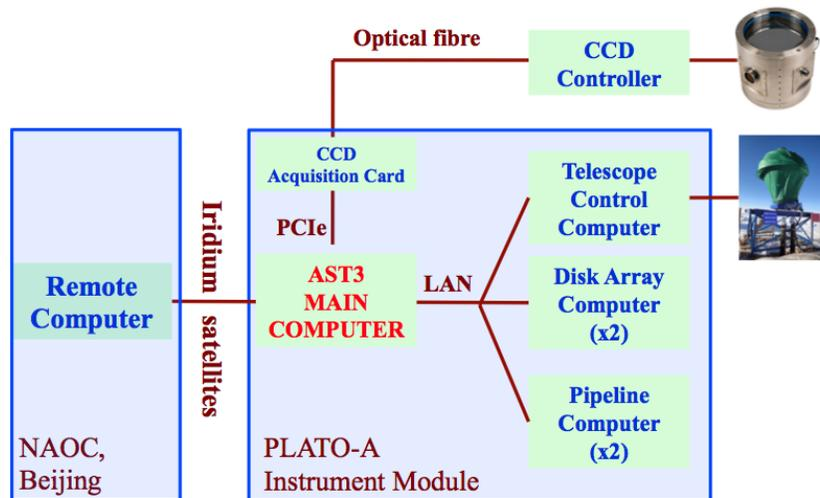
Figure 1. Schematic diagram of the AST3 operation system.
