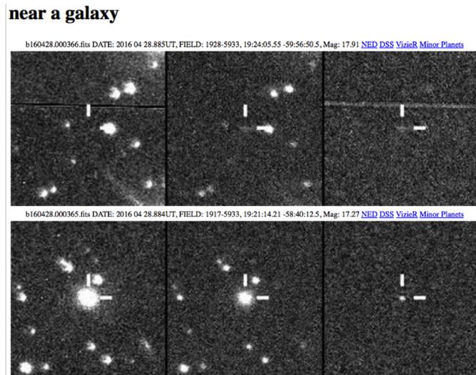
Figure 2. Two examples of the transient candidates on the website. The stamp images are, from left to right, template image, observed image, and difference image showing the detected transient. Listed on top of each candidate are image file name, observing date and time, field name, RA, Dec, magnitude of the transient, as well as links to other astronomical databases for easy comparison and visual check.
