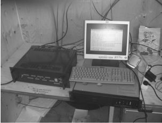
Figure 10: (left) The Supervisor computer of the Gattini cameras provides fully automated control of the instruments during the year, including temperature monitoring and Iridium connection to Sydney for data and status download. A UPS is included to provide a safe method for shutdown if and when station power recycles.
