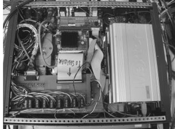
Figure 10: (left) The Supervisor computer of the Gattini cameras provides fully automated control of the instruments during the year, including temperature monitoring and Iridium connection to Sydney for data and status download. A UPS is included to provide a safe method for shutdown if and when station power recycles.
