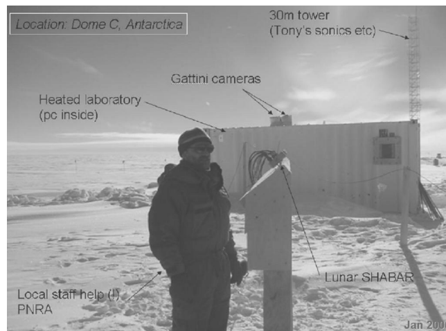
Figure 2: The Gattini cameras are located on the roof of the atmospheric laboratory at the Dome C site as shown above. The laboratory is a heated environment, a requirement for the control computer. The 30m tower shown in the background is used for ground layer profiling. In the foreground a transit lunar shabar points northwards.
