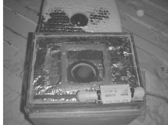
Figure 16: (left) The newly installed Gattini cameras inside their respective insulated enclosures on the roof of the atmospheric laboratory at Dome C. The Gattini-SBC window suffered icing problems from May onwards.
