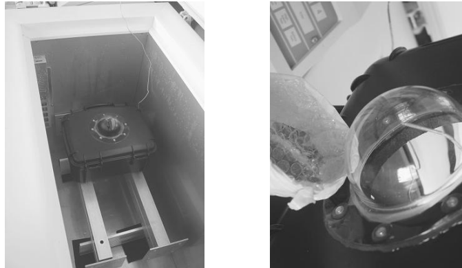
Figure 13: (left) A camera enclosure under low temperature testing. The biological fridge provided a temperature range from ambient (in Sydney) to -80^{\circ}\text{C} , quite adequate for the ambient temperatures expected at the Dome C site.
