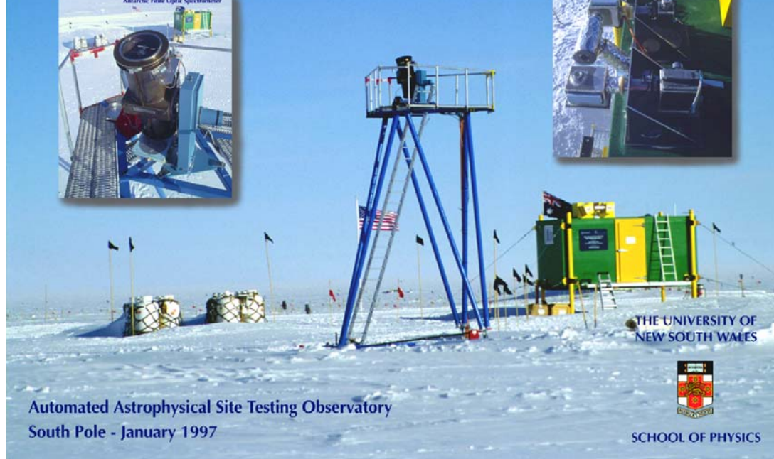
Figure 3: The AASTO at the South Pole. The shelter is to right and the fuel supply to left. The tower, at centre, supports a 30-cm telescope. The two insert pictures show three of the experiments, a UV/optical fibre-optic spectrometer to left (attached to the 30-cm telescope) and near- and mid-infrared sky brightness monitors to right.
