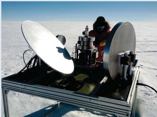
Antarctic HEAT. (a) Craig Kulesa installs the HEAT (High Elevation Antarctic Terahertz) telescope at Ridge A in January 2012. Light bounces off the flat primary siderostat (rotatable) mirror onto the 0.6-m-aperture parabolic mirror at right. From there it is directed into an ellipsoidal tertiary that finally shunts it to a detector in the cryostat next to Kulesa. (Photo by Luke Bycroft.) (b) In this January 2012 scene at Ridge A, the HEAT telescope is to the left, sitting on stilts and protected by a terahertz-transparent material. The other objects are elements of the PLATO-R observatory. The yellow box is the instrument module, and the black object at right is a solar-panel array, which comprises eight 195-W panels arranged in a cube. On the roof of the instrument module sit various satellite antennas, web cameras, and an all-sky camera called HRCAM3. The blue-and-white flag is that of the Scientific Committee on Antarctic Research. The engine module that provides power when the Sun is down is 60 m away. (Photo by Craig Kulesa.)
