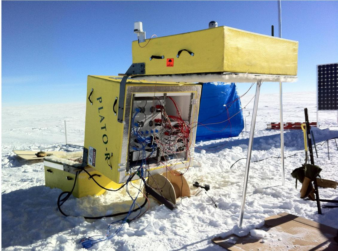
Figure 4: The PLATO-R Instrument Module at Ridge A, hinged open for easy access to the battery pack at left, the electronic racks in the center, and the lid containing the Iridium aeriels and cameras. The thick black “umbilical” cable connects the Instrument Module with the Engine Module; it contains two 120 VDC copper wires, an earth wire, and a Controller Area Network cable. Solar panels are visible to the right. The tarpaulin to the right of center was used as a wind break during assembly.
