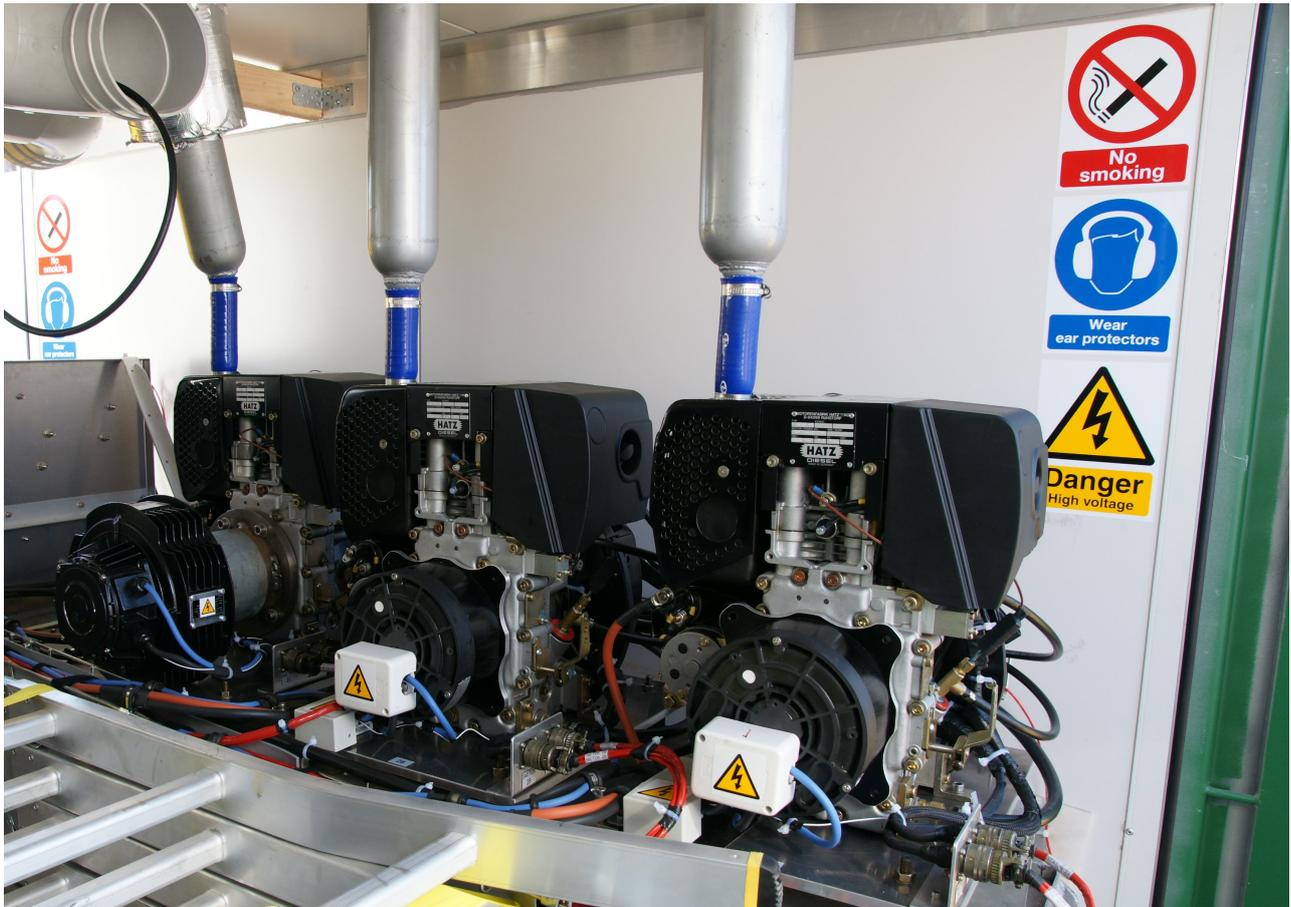
Figure 3. A view inside the PLATO Engine Module, prior to the original deployment in January 2008. Three of the six Hatz diesel engines are visible. The new design will place the exhaust tubes out the side rather than the top. The high-current starter motor wiring will be eliminated. The engines will be on modular, easily-replaceable, plates.
