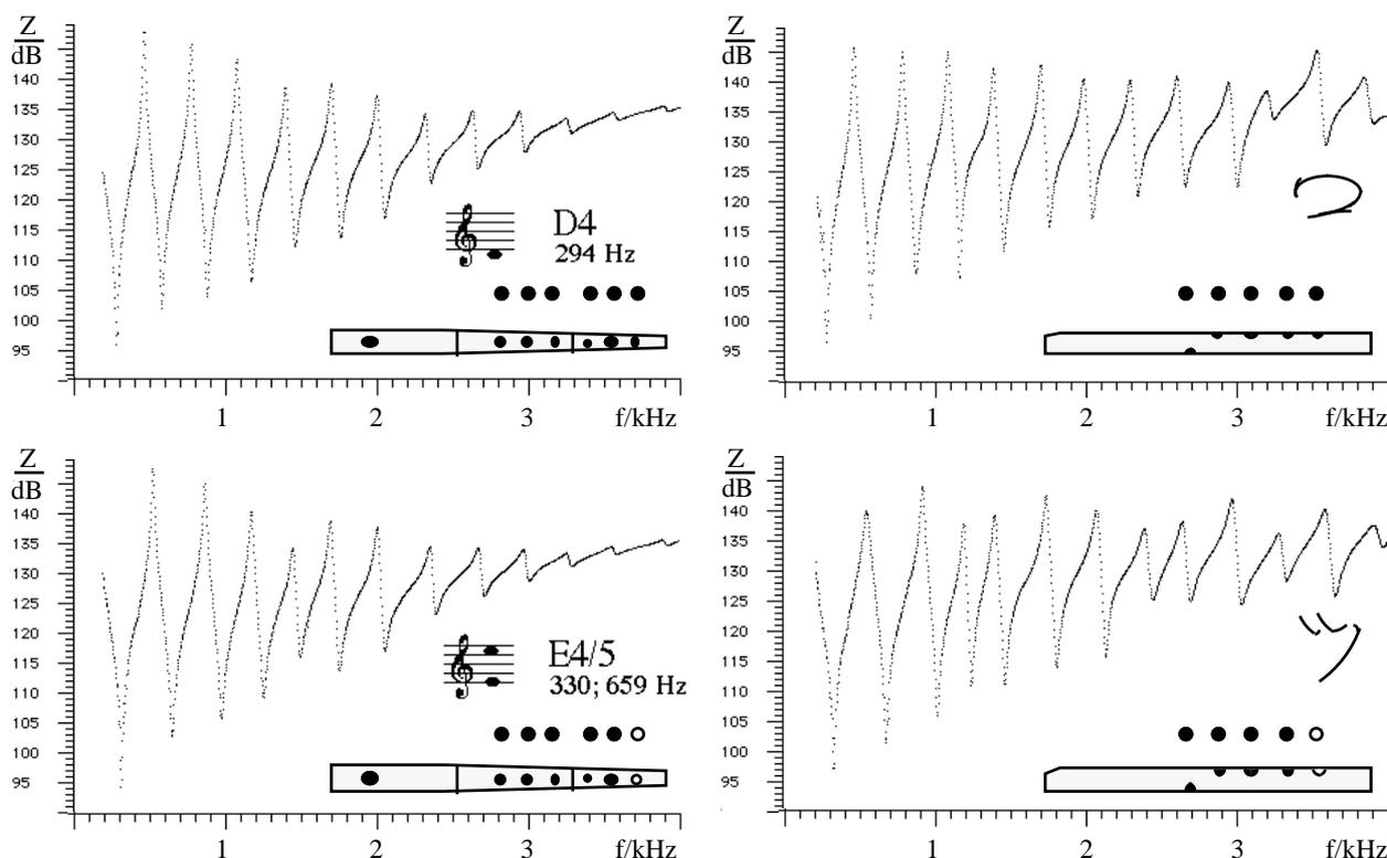
**Fig. 2** Impedance spectra for the two lowest notes on the flute (left) and the shakuhachi (right)
