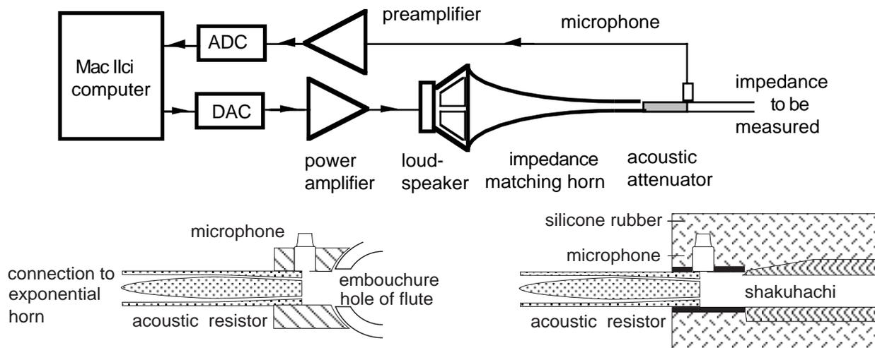
**Fig. 1** Schematic of the acoustic impedance spectrometer (top) and measurement geometries for the flute (bottom left) and shakuhachi (bottom right). Figure is not to scale.
