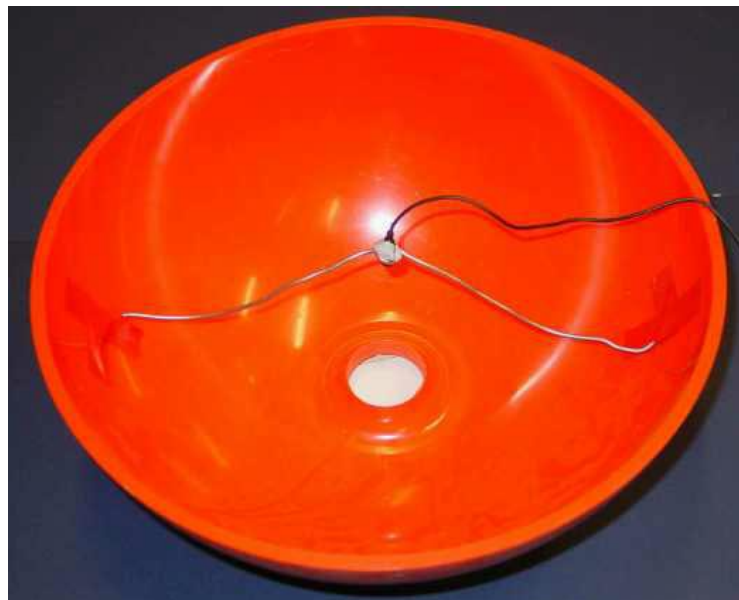
A directional mic made from half a fishing buoy, a piece of wire and a lapel microphone.
