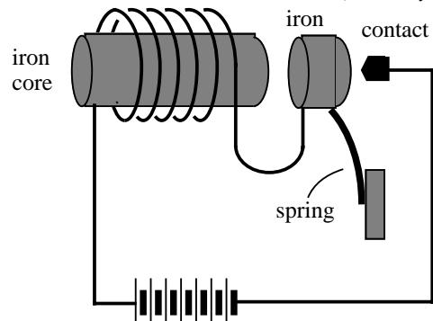
spring moves iron right to close contact.  $i$  flows which causes  $\mathbf{B}$
