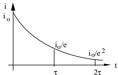
iii) switch at b for long time ( $i = 0$ ). Switch to a at  $t' = 0$ .
