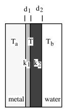
A large, metal object is maintained at constant, uniform temperature  $T_a$ . It is coated with two uniform, thin layers of insulating material. The first coat has thickness  $d_1$  and thermal conductivity  $k_1$ . The second coat has thickness  $d_2$  and thermal conductivity  $k_2$ . The coated metal object is immersed in water at constant, uniform temperature  $T_b$ . A section of the object and coatings is shown in the sketch.
