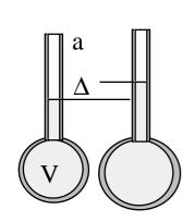
The diagram shows a fluid-in-glass thermometer at two different temperatures: T and T +  $\Delta$ T. The fluid has a coefficient of thermal expansion  $\beta_f$  and the glass has a coefficient of thermal expansion  $\beta_g$ , which is less than  $\beta_f$ , but which is not zero. The volume of the cylindrical part is very much smaller than that of the spherical part. When the temperature rises by  $\Delta$ T, the liquid rises  $\Delta x$  in the cylindrical part of the thermometer, as shown.
