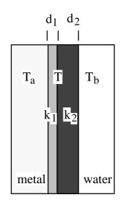
A large, metal object is maintained at constant, uniform temperature  $T_a$ . It is coated with two uniform, thin layers of insulating material. The first coat has thickness  $d_1$  and thermal conductivity  $k_1$ . The second coat has thickness  $d_2$  and thermal conductivity  $k_2$ . The coated metal object is immersed in water at constant, uniform temperature  $T_b$ . A section of the object and coatings is shown in the sketch.
