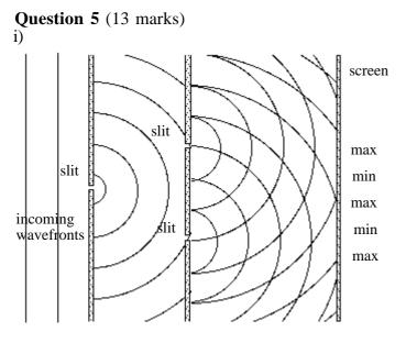
e.g. Young's experiment. Light passes through one slit (gives *coherent source*) then two slits. This gives an interference pattern on a screen. Waves arriving in phase give interference maxima, those arriving out of phase produce destructive interference. Interference is a phenomenon characteristic of waves.
