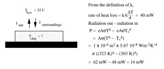
ii) Put a (thermally conducting but electrically insulated) heat sink on top of the chip. This conducts heat away and then loses it by radiation, or (if connected) by conduction to the existing heat sink.
