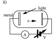
e.g. The photoelectric effect. The apparatus uses a variable potential difference to turn back ejected electrons, and thus to measure their energy. Electrons are ejected by photons as soon as the metal electrode is exposed, whatever the intensity. The energy of an ejected electron depends on the wavelength, but not on the intensity. This suggests interaction with a single electron and therefore localisation. Localisation of energy in a collision is characteristic of particles.
