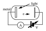
e.g. The photoelectric effect. The apparatus uses a variable potential difference to turn back ejected electrons, and thus to measure their energy. Electrons are ejected by photons as soon as the metal electrode is exposed, whatever the intensity. The energy of an ejected electron depends on the wavelength, but not on the intensity. This suggests interaction with a single electron and therefore localisation. Localisation of energy in a collision is characteristic of particles.
