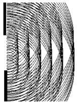
Use Huygen's construction: beam of finite width, interference if  $d\sim\lambda$
