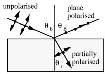
When refracted ray  $\bot$  reflected  $\to$  plane polarised reflected wave (Brewster's angle  $\theta_B$ ).
