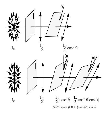
**Example**. Two crossed polarisers (polar<sup>n</sup> dir<sup>n</sup> are at right angles) have a third polariser between them. What is the transmitted intensity? What angle for the middel polariser gives
