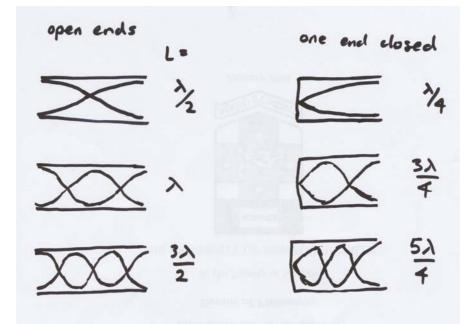
10. The difference in distance between the two resonances should correspond to half a wavelength of the waves. That is  $\frac{\lambda}{2} = 0.683 - 0.228 = 0.455 m$ , and the wavelength of the waves is then  $\lambda = 0.91 m$ . The speed of the sound is then  $v = f\lambda = 384 \times 0.91 = 350 m s^{-1}$ . The next resonance will occur a further half wavelength along, at 68.3 + 45.5 = 114 cm.
