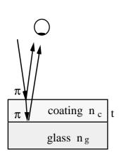
If the film has a value of refractive index intermediate between that of the glass and that of the external medium, then there will be a phase change of  $\pi$  at the two reflections shown. For normal incidence, these two rays will have a phase difference of  $\pi$  if
