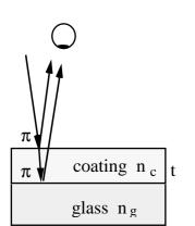
If the film has a value of refractive index intermediate between that of the glass and that of the external medium, then there will be a phase change of  $\pi$  at the two reflections shown. For normal incidence, these two rays will have a phase difference of  $\pi$  if
