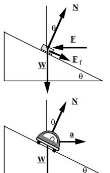
No acceleration so  $\Sigma$  forces = 0. Resolve forces in i) 1 the directions normal to and in the plane.  $N = W\cos\theta + F\sin\theta$ In the normal: In the plane  $F\cos\theta = W\sin\theta + F_f$ .  $F\cos\theta = W \sin\theta + \mu_k N$
