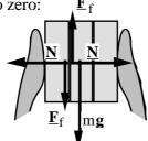
Bricks not accelerating horizontally, so normal force from hands = normal force between bricks.
