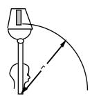
**Example.** Foolhardy lecturer swings a bucket bricks in a vertical circle. How fast should he swing so that the bricks stay in contact with the bucket at the top of the trajectory?
