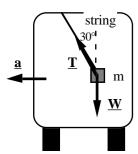
We know: tension in direction of string, weight down, acceleration horizontal circular motion
