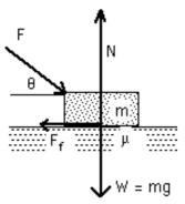
Apply force F at  $\theta$  to horizontal. Mass m on floor, coefficients  $\mu_s$  and  $\mu_k$ . For any given  $\theta$ , what F is required to make the mass move? Eliminate 2 unknowns N and  $F_f \rightarrow F(\theta, \theta)$
