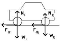
**Example.** Rear wheel drive car, 300 kg wt on **each** front wheel, 200 kg wt on rear. Rubber-road:
