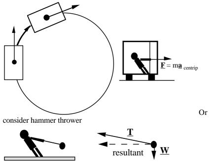
Resultant force produces acceleration in the horizontal direction, towards the centre of the motion
