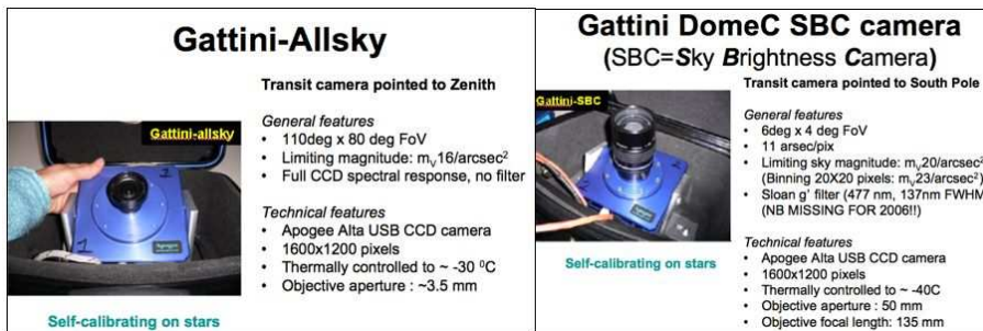
Fig. 1. The specifications for the Gattini cameras are shown for the wide field all-sky camera (left); and for the larger aperture narrow field camera (right).
