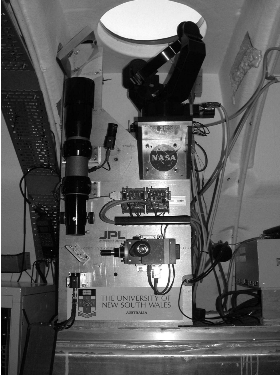
Fig. 1. The MASS instrument, telescope and siderostat, as installed in the AASTINO, February 2004
