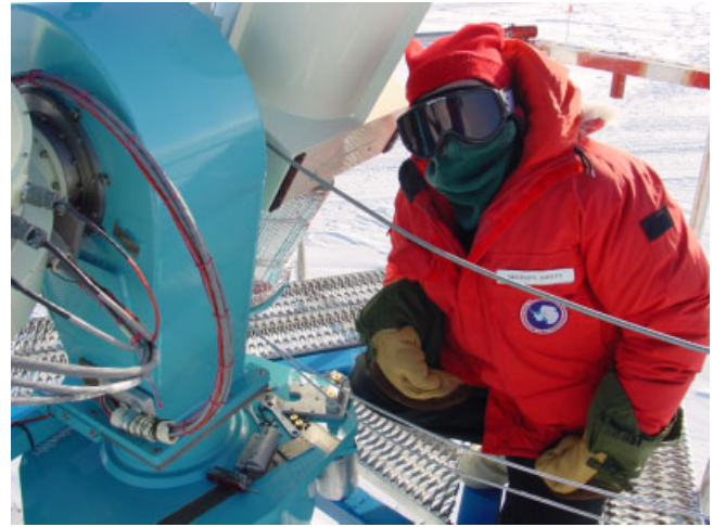
Fig. 5. (online colour at www.an-journal.org ) Telescopes should be designed for maintenance at low temperatures.
