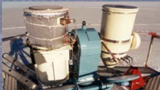
A-DIMM (right) installed at the South Pole on the G-mount. The instrument on the left is the AFOS
