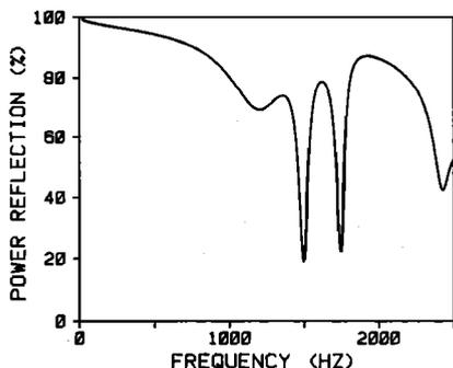
FIG. 7. Calculated power reflection coefficient for closed D# key fingering of  $A_6$ .
