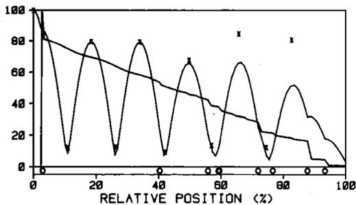
FIG. 6. Calculated pressure and power distributions in flute bore when fingered for  $A_6$  with closed D# key. Resonance frequency was 1800 Hz.
