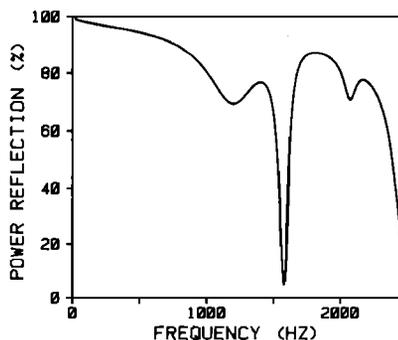
FIG. 5. Calculated power reflection coefficient looking into open hole portion of bore at  $C\#$  hole for open  $D\#$  key fingering of  $A_6$ .
