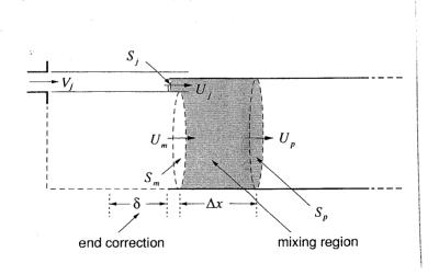
4. Assumed geometry for calculation of the interaction of a jet, with varying deflection, and a pipe resonator. [Fletcher]
