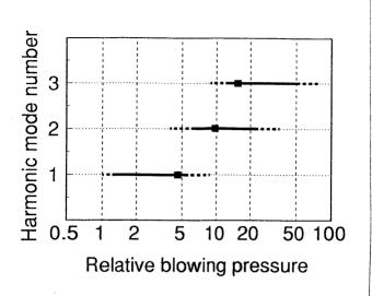
6. Ranges of relative blowing pressure over which the first three modes of an open pipe can be excited by an air jet. The actual blowing pressures depend on the jet length and pipe length. Square symbols indicate values of blowing pressure necessary to achieve reliable single-mode excitation.
