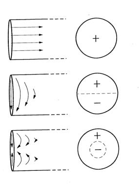
13. The plane wave mode (upper figure) and two evanescent higher modes in a circular pipe.
