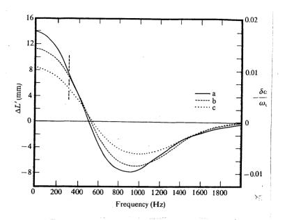
16. Variation with frequency of the total end-correction  $\Delta L'$  of a flute head joint, as affected by head taper. [Benade and French]
