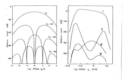
10. Calculated and measured dependence of harmonic levels on jet offset for an organ pipe.
