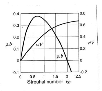
2. Approximate behavior of the amplification factor  $\mu$  and wave velocity  $\nu$  on a jet of half-width b and central velocity V. [Thwaites and Fletcher]
