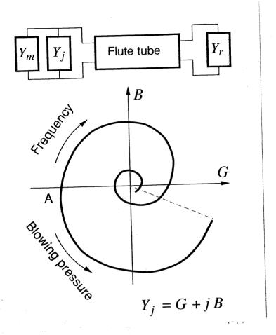
5. Assumed network for interpreting the admittance behavior of an air jet interacting with a flute tube, and the resulting generalized admittance behavior. [Thwaites and Fletcher]
