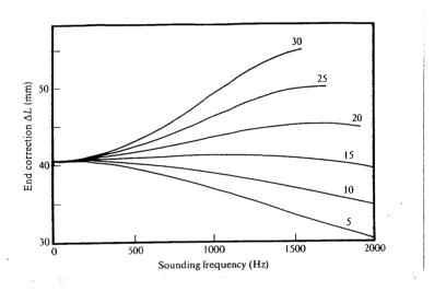
15. Variation with frequency of the end-correction  $\Delta L$  at a flute embouchure, as affected by the position of the stopper, shown in millimeters distance from the center of the embouchure hole. [Fletcher and Rossing]
