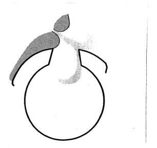
17. Cross-sectional view of the embouchure hole of a metal flute, showing the undercut chimney.
