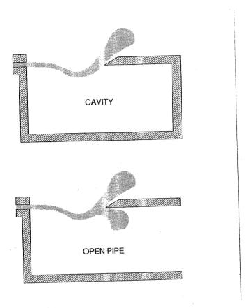
3. Contrasting behavior of an air jet exciting a closed cavity and an open pipe. In the former case the jet appears to re-attach to the lip so that there is no jet flow into the cavity.
