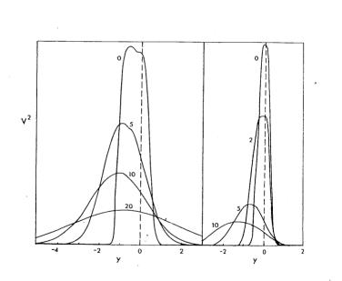
11. Variation of the jet velocity profile (displayed as the square of the velocity) as a function of distance from the flue (given in millimetres) for two jets. In the left-hand figure the flue width is 1 mm, while in the right-hand figure it is 0.25 mm. [Fletcher]
