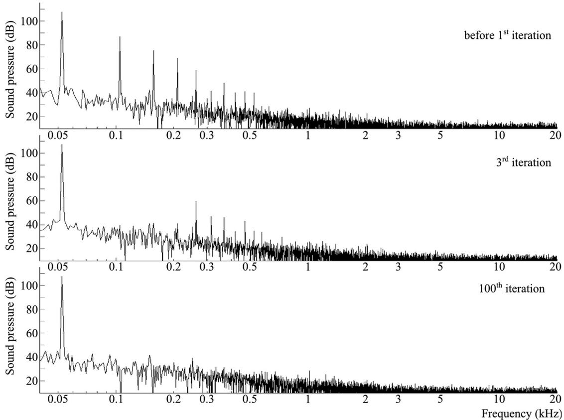
FIG. 1. The reduction of harmonic distortion by successive iterations. (a) The sound pressure spectrum (in dB with respect to  $20 \mu\text{Pa}$ ) recorded by the microphone when a pure sine wave at 52.49 Hz was input to the distorting system. (b) The result after three iterations. (c) After 100 iterations, all harmonics in the audible range have been reduced to  $>65$  dB below the fundamental. (The small peaks at 150 and 250 Hz are harmonics of mains interference, not harmonics of the signal.)
