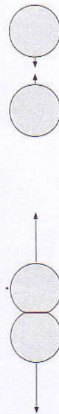
Figure 5.19. When two molecules come very close together they repel each other strongly. When they are a short distance apart they attract each other.
