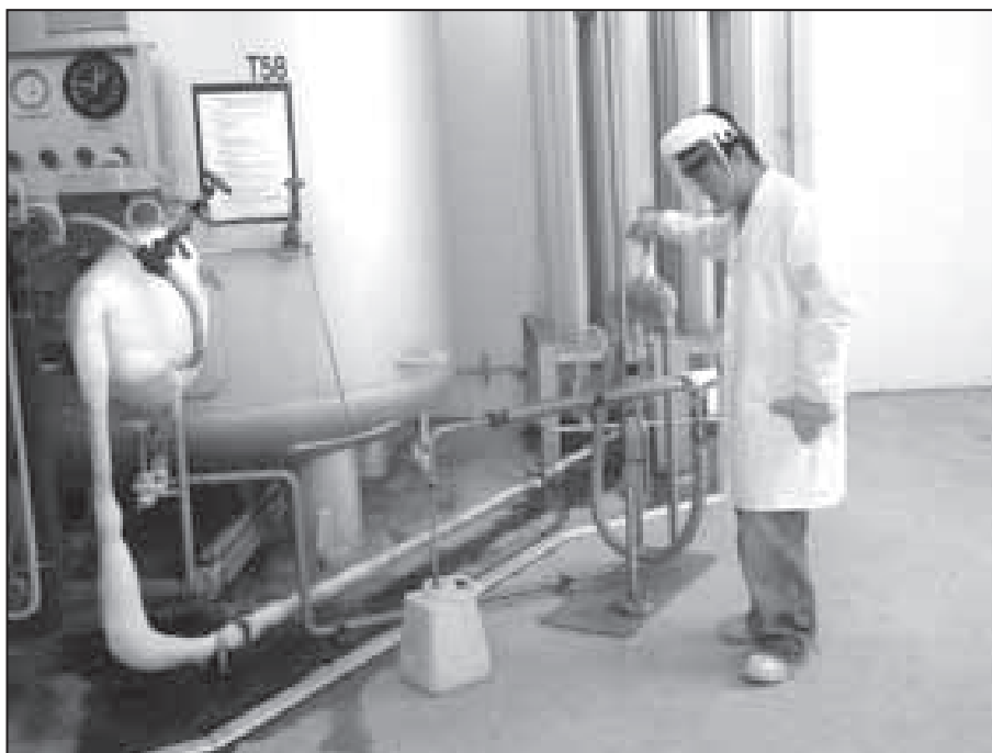
An undergraduate physics student wearing the correct protective gear and demonstrating a safe way to dispense liquid nitrogen.
