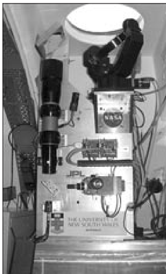
The Multi-Aperture Scintillation Sensor installed in the UNSW AASTINO facility at Dome C, Antarctica.
